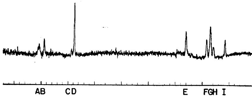
Figure 5. NMR Spectrum of Organic Fluorocompound(s) Isolated from Human Plasma
