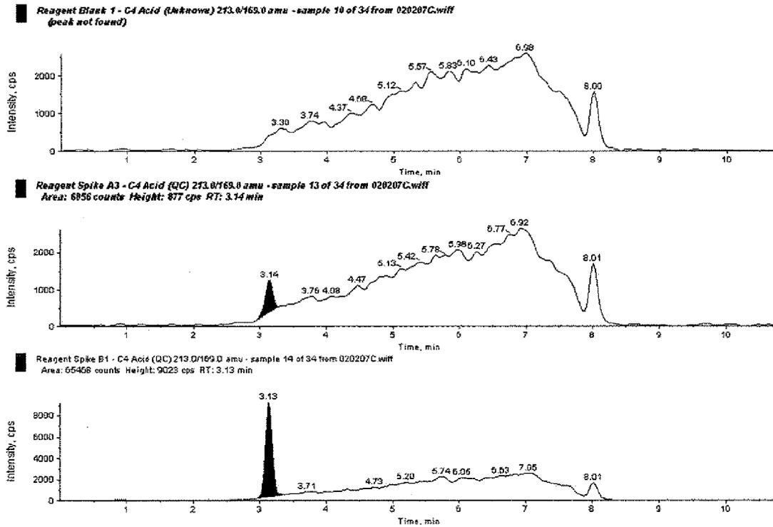
**Figure 6. Chromatogram Representing a Water Sample Analyzed for PFBA (Exygen ID: C0225143, Data Set: 020207C)**
