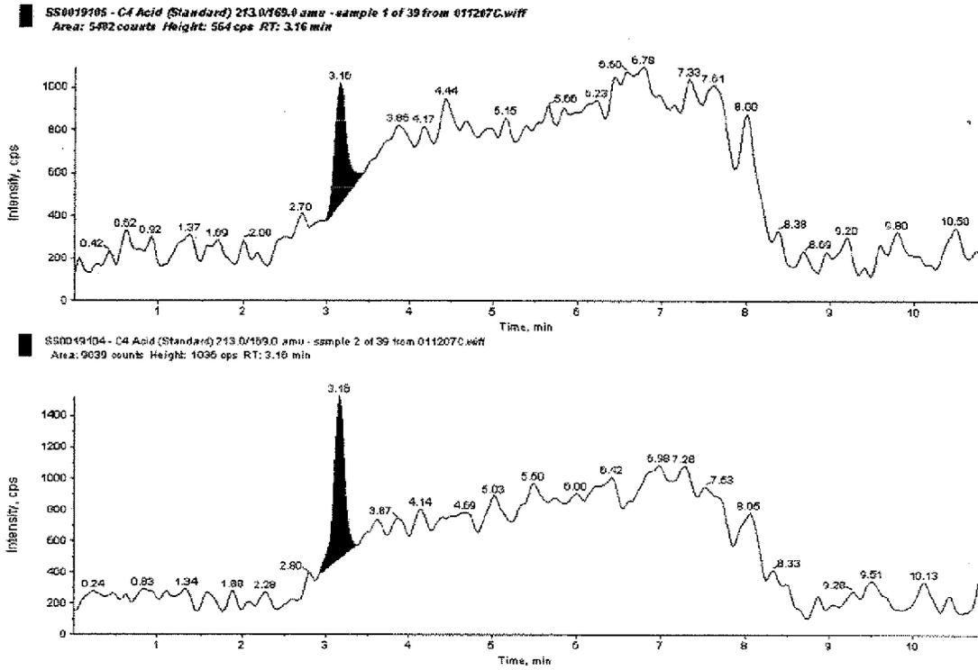
**Figure 3. PFBA in a Control Blank, a 2.0 ng/g Fortified Control Spike A, and a 20 ng/g Fortified Control Spike B, Respectively**
