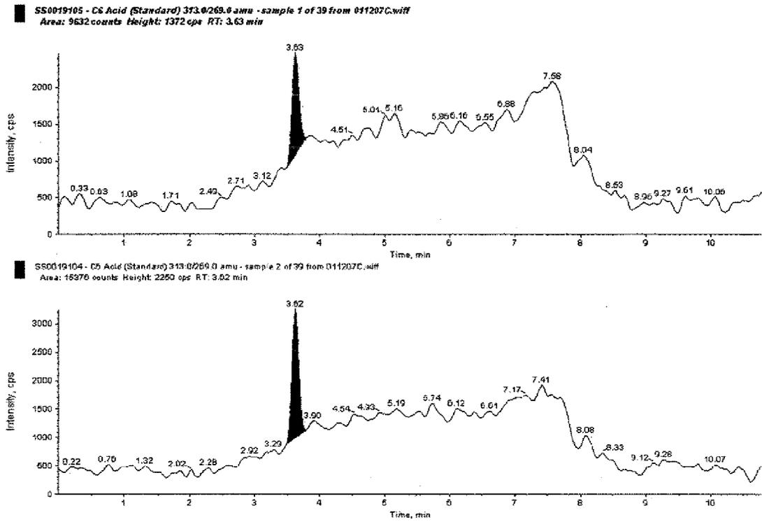
**Figure 15. PFHA in a Control Blank, a 2.0 ng/g Fortified Control Spike A, and a 20 ng/g Fortified Control Spike B, Respectively**
