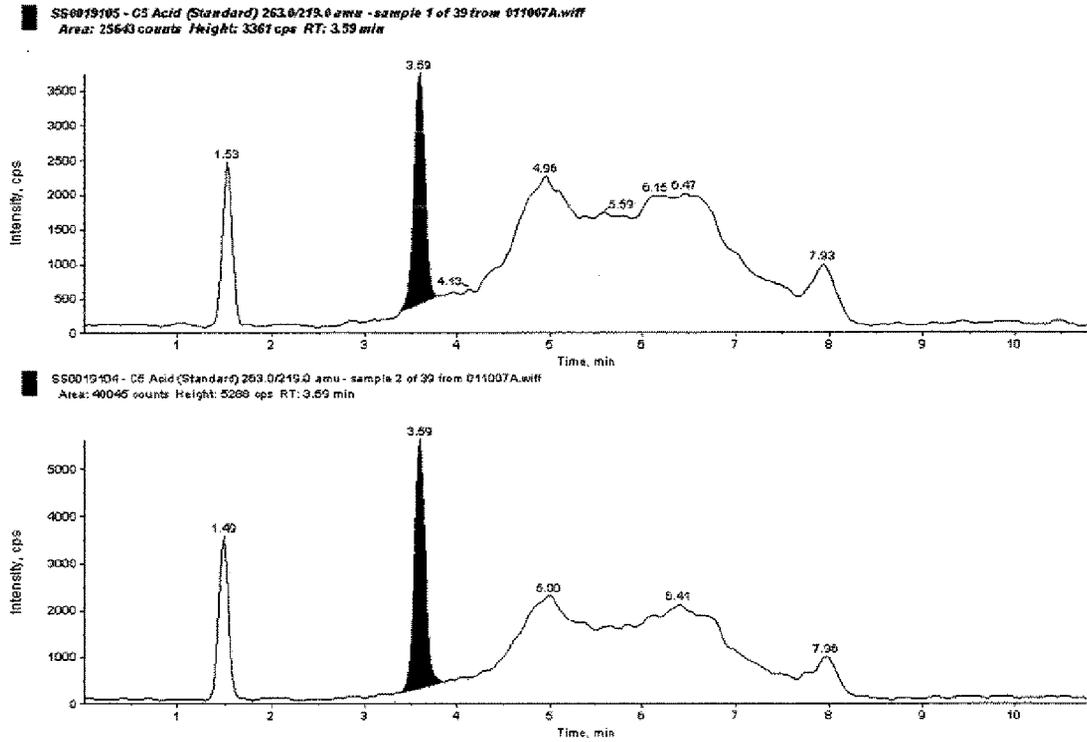
**Figure 9. PFPeA in a Control Blank, a 2.0 ng/g Fortified Control Spike A, and a 20 ng/g Fortified Control Spike B, Respectively**
