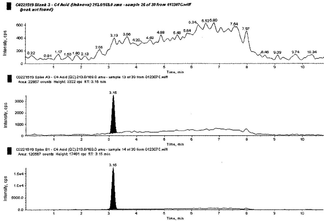
**Figure 4. Chromatogram Representing a Soil Sample Analyzed for PFBA (Exygen ID: C0225092, Data Set: 011207A)**
