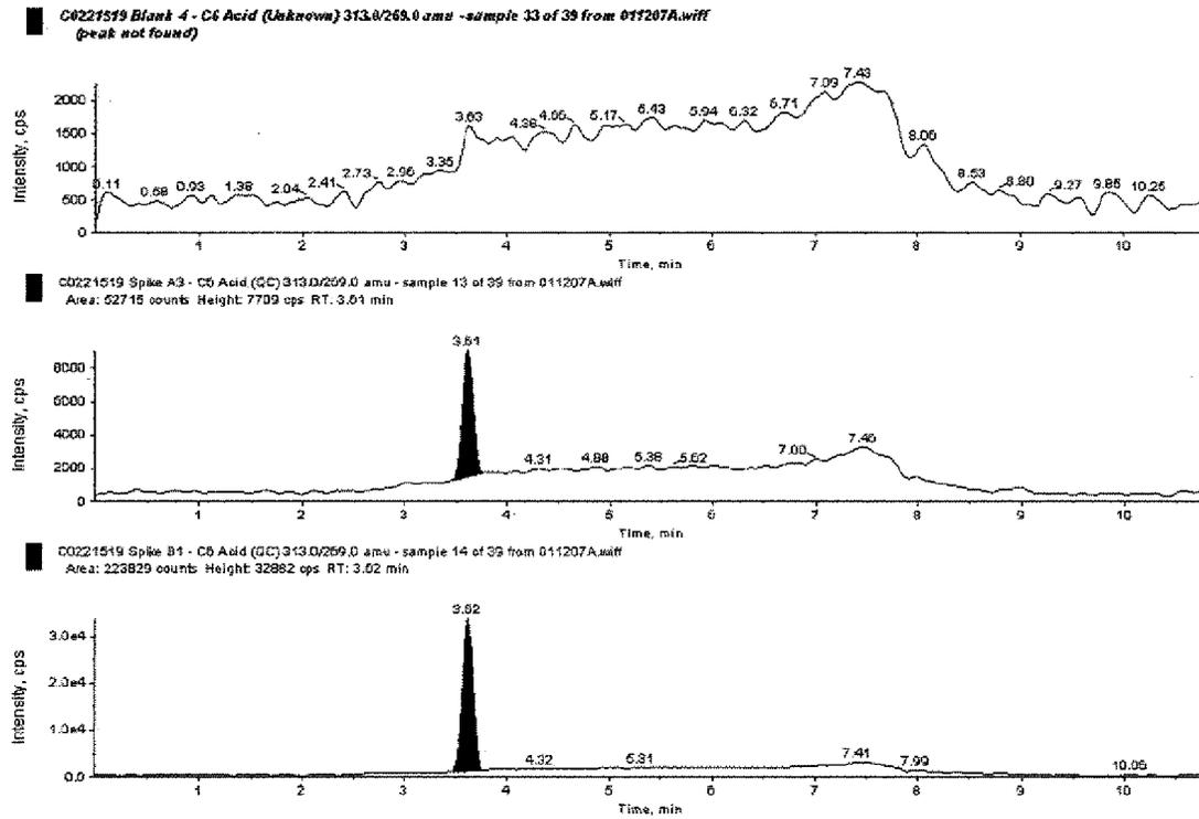
**Figure 16. Chromatogram Representing a Soil Sample Analyzed for PFHA (Exygen ID: C0225092, Data Set: 011207A)**
