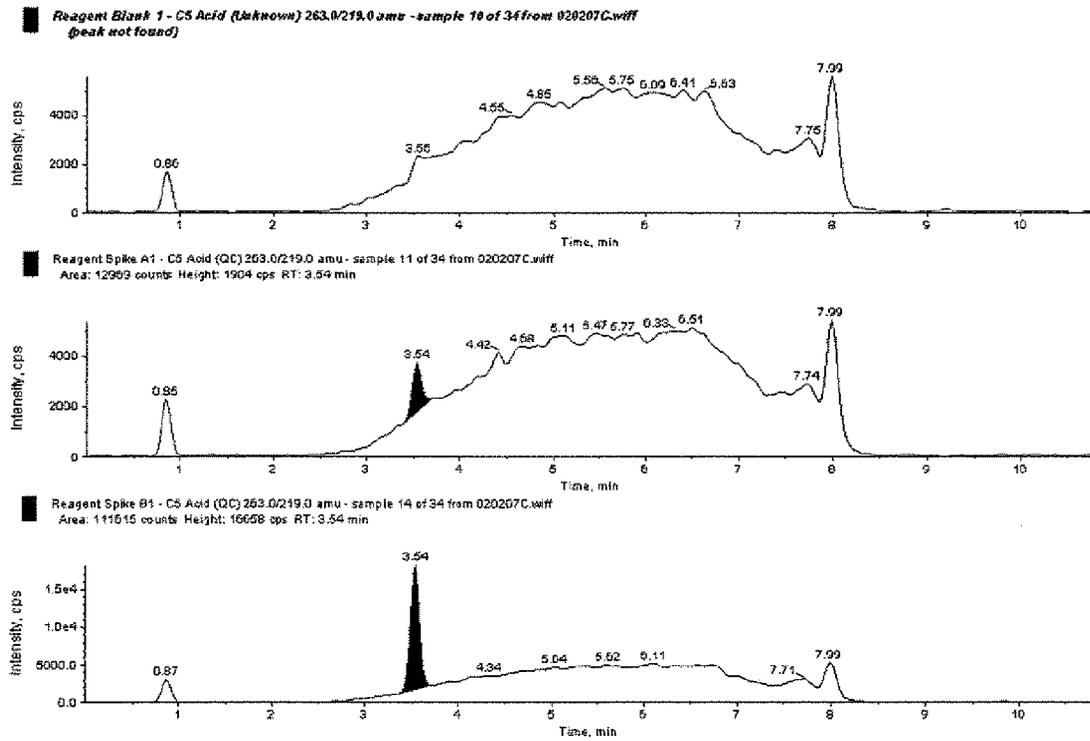
**Figure 12. Chromatogram Representing a Water Sample Analyzed for PFPeA (Exygen ID: C0225101, Data Set: 020207C)**
