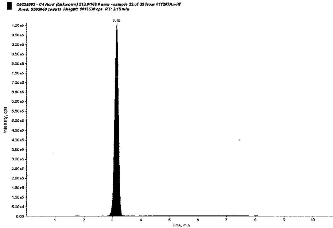
**Figure 5. PFBA in a Reagent Blank, a 0.25 ng/mL Fortified Reagent Spike A, and a 2.5 ng/mL Fortified Reagent Spike B, Respectively**
